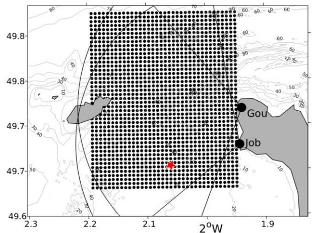
**Figure 1 :** Map showing the radar stations at Goury (Gou), and Jobourg (Job), their maximum coverage for wave measurement (black arcs), and measuring grid (black dots). The red star indicates the position where the ADCP was deployed. The latitude is degrees North, and the longitude degrees West.
