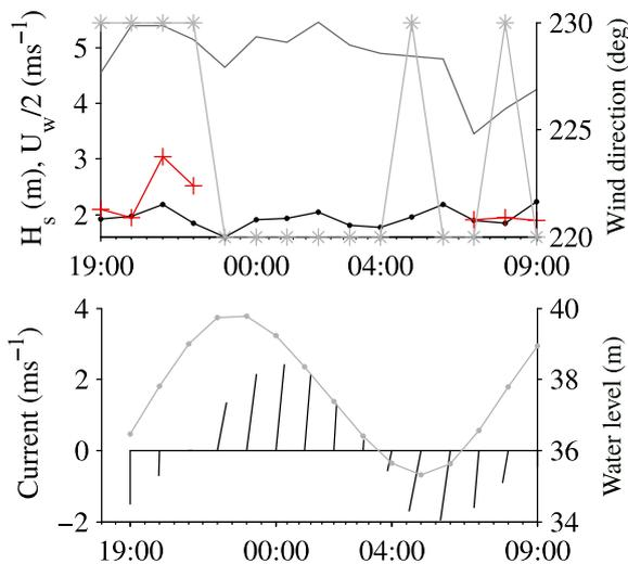
**Figure 2:** The top panel shows the significant wave height measured by the ADCP (black line and dots), and by the radar (red line and cross). The 10 m wind speed (grey line) and direction (grey and star), measured at a meteorological station at Goury are also shown. The lower panel shows the water level as measured by the ADCP (grey line and dots), and the current vectors measured by the radars (black lines).
