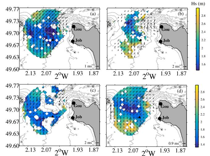
**Figure 5.** Maps of significant wave height (colour) and surface current (vectors) measured by the radar on (a) 24 January 2018 at 19:00, (b) 24 January 2018 at 22:00, (c) 25 January 2018 at 08:00, (d) 25 January 2018 at 09:00. The latitude is degrees North, and the longitude is degrees west. The colorbar indicates  $H_s$  in meters. The reference arrow represents the maximum current velocity measured.
