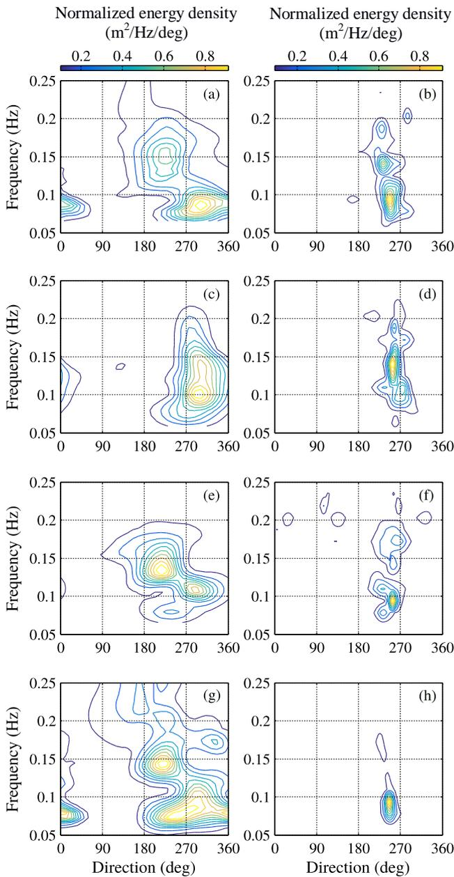
**Figure 4:** Wave directional spectra measured by the radar (left) and the ADCP (right). (a, b) 24 January 2018 at 19:00, (c, d) 24 January 2018 at 22:00, (e, f) 25 January 2018 at 08:00, (g, h) 25 January 2018 at 09:00. The colour scale represents the energy density normalized by the maximum of the spectrum. The contours are plotted at levels between 0.1 and 0.9, every 0.1  $\text{m}^2/\text{Hz}/\text{deg}$ .
