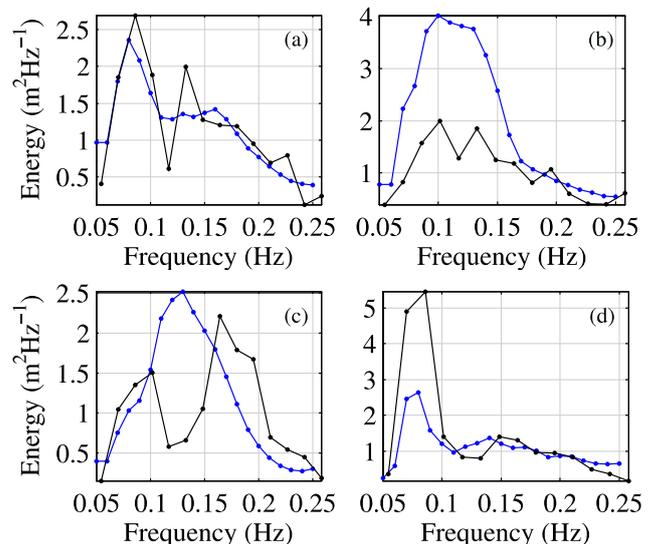
**Figure 3:** Wave spectra measured by the ADCP (black) and the radar at four different times through a tidal cycle. (a) 24 January 2018 at 20:00, (b) 24 January 2018 at 22:00, (c) 25 January 2018 at 08:00, (d) 25 January 2018 at 09:00. Note the different resolution of the two types of spectra: 0.015 Hz (ADCP), 0.01 Hz (radar).
