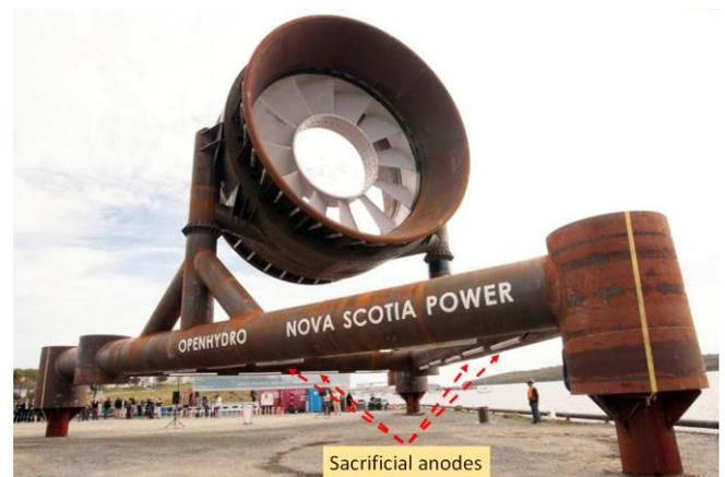
**Figure 3:** OpenHydro support structure with sacrificial anodes, weigh of each foundation ~400 tons (turbine fixed to the seabed via gravity only) [18].
