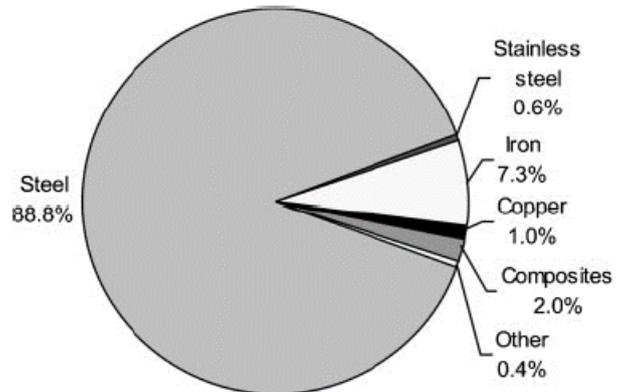
**Figure 4:** Materials used in the manufacture of the SeaGen turbine [32].
