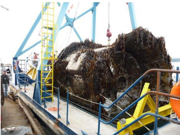
**Figure 3:** Biofouling on TidGen turbine deployed in Eastport, Maine in North America (2007) [3].
